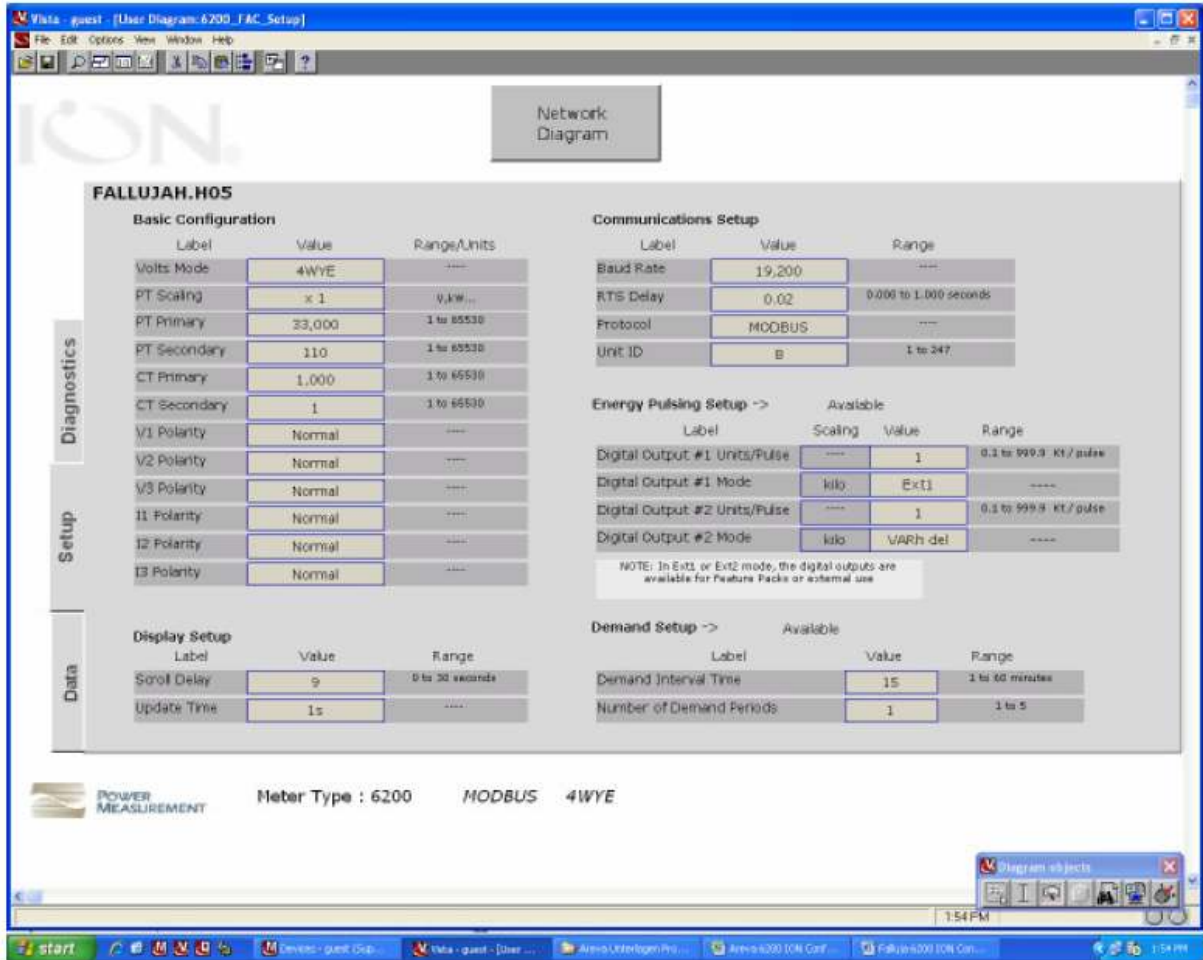
Fig. (9): Setting parameters to the ION 6200 meter (H5, incoming 33KV)
