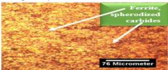
Figure 3. base- metal zone for AISI 420 MSS after annealing at 850°C/15 min.
