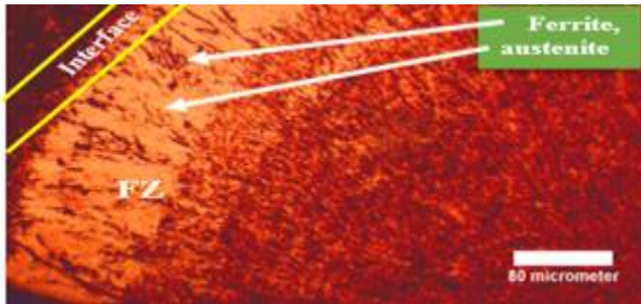
Figure 2. Fusion- metal zone for AISI 420 MSS/ ER 399L after annealing at 850°C/15 min.
