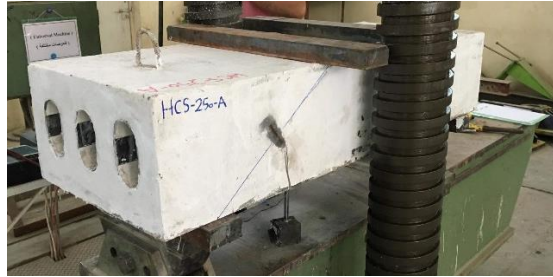
Figure 6. The HCS Specimen in the Machine Test
