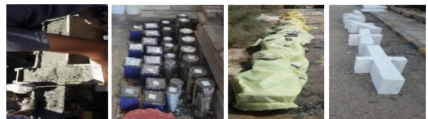
Figure 6: Casting and Curing of RCASCC Beams.
