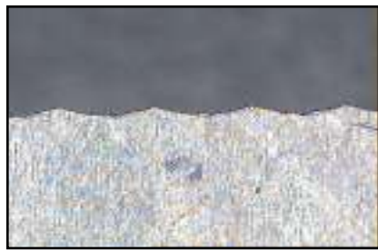
(a) Pick-interval scallop height.
