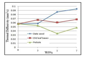
Fig. 7: The effect of filler (type and weight fraction) on the thermal diffusivity.
