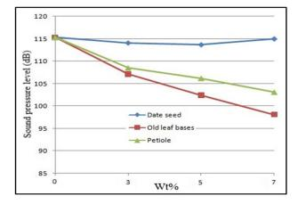
Fig. 9: Effect of filler content and type on the sound pressure level at 100 HZ frequency.
