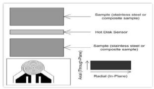
Fig. 1: The Schematic of Hot disk sensor.
