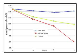
Fig. 10: Effect of filler content and type on the sound pressure level at 6 kHZ frequency.
