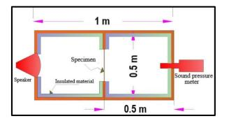
Fig. 5: The sound-insulated box.
