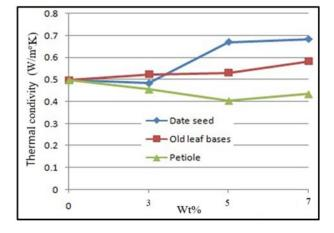
Fig. 6: The effect of filler (type and weight fraction) on the thermal conductivity.
