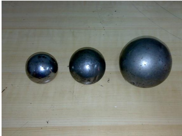
(a) Bearing Balls as dies.
