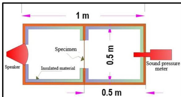
Fig. 5: The sound-insulated box.
