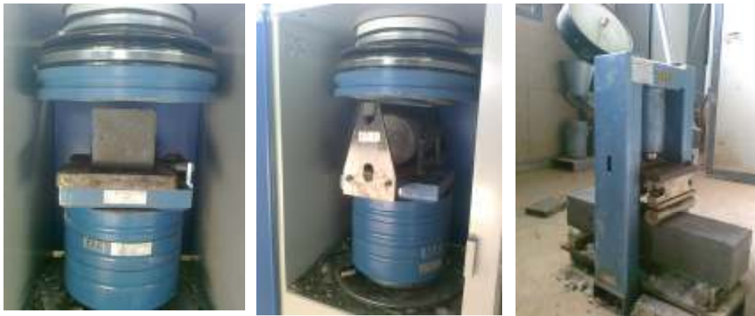
Figure (9): Specimens inside the testing machine during test.
