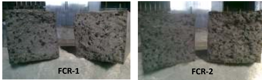
Figure (8): Crumb rubber distribution through specimens.
